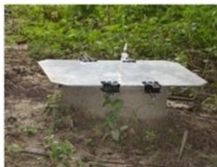
**Figure 2: A static chamber measuring N<sub>2</sub>O and CH<sub>4</sub> fluxes on an oil palm plantation near Lahad Datu, Borneo. The chamber is sealed for 60 minutes. Air samples were withdrawn at intervals and sent to CEH, Edinburgh for analysis by gas chromatography.**
