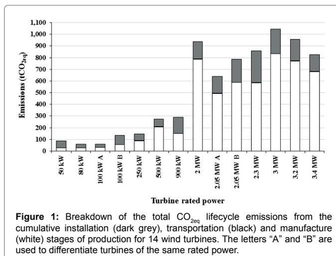
**Figure 1:** Breakdown of the total CO<sub>2eq</sub> lifecycle emissions from the cumulative installation (dark grey), transportation (black) and manufacture (white) stages of production for 14 wind turbines. The letters “A” and “B” are used to differentiate turbines of the same rated power.
