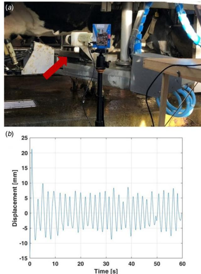
**Fig. 4.** Use of micro-Doppler radar for detecting respiration and heart rate. **Figure 4a** shows the radar equipment positioned within a milking robot. **Figure 4b** shows the micro-Doppler phase signal indicating motion of chest wall as a result of breathing.
